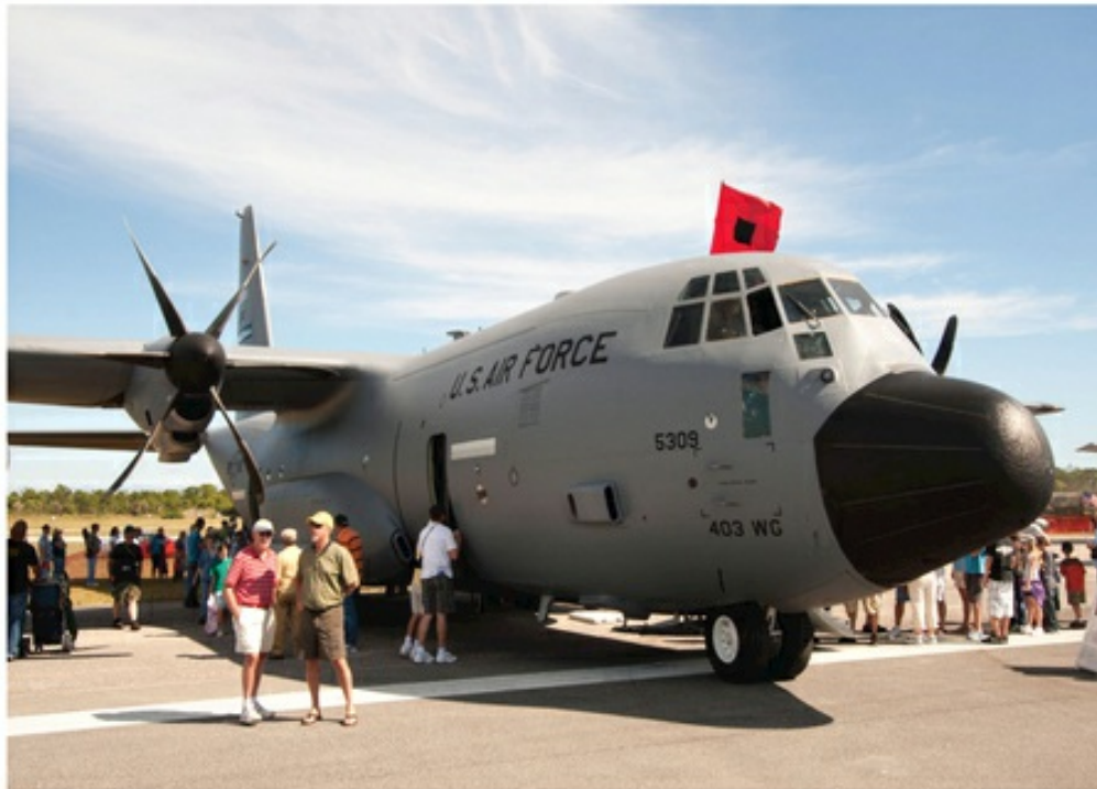
FIGURE 10.4.A Hurricane Hunter Aircraft This U.S. Air Force Reserve Lockheed Martin WC-130 aircraft, based at Kessler Air Force Base in Mississippi, is specially equipped for taking weather measurements in hurricanes. WC-130 aircraft similar to this one investigate hurricanes at the direction of the National Hurricane Center. (Patrick Phelan/Alamy Stock Photo)
