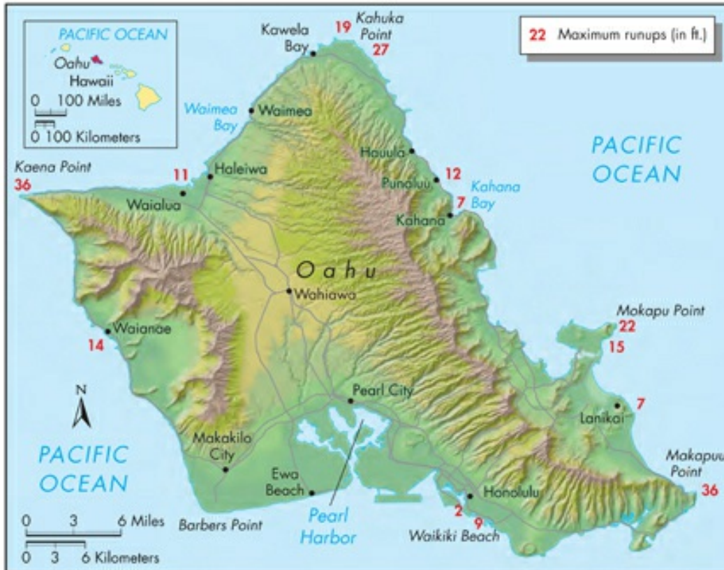
FIGURE 4.17 Tsunami Runup on Oahu, Hawaii Map of Oahu showing runup of the 1946 tsunami that originated from an earthquake in the Aleutian Islands, Alaska. Maximum runups are indicated in feet. (Based on Walker, D., "Tsunami Facts," SOESTechnical Report 94-03, School of Ocean and Earth Science and Technology, 1994.)
