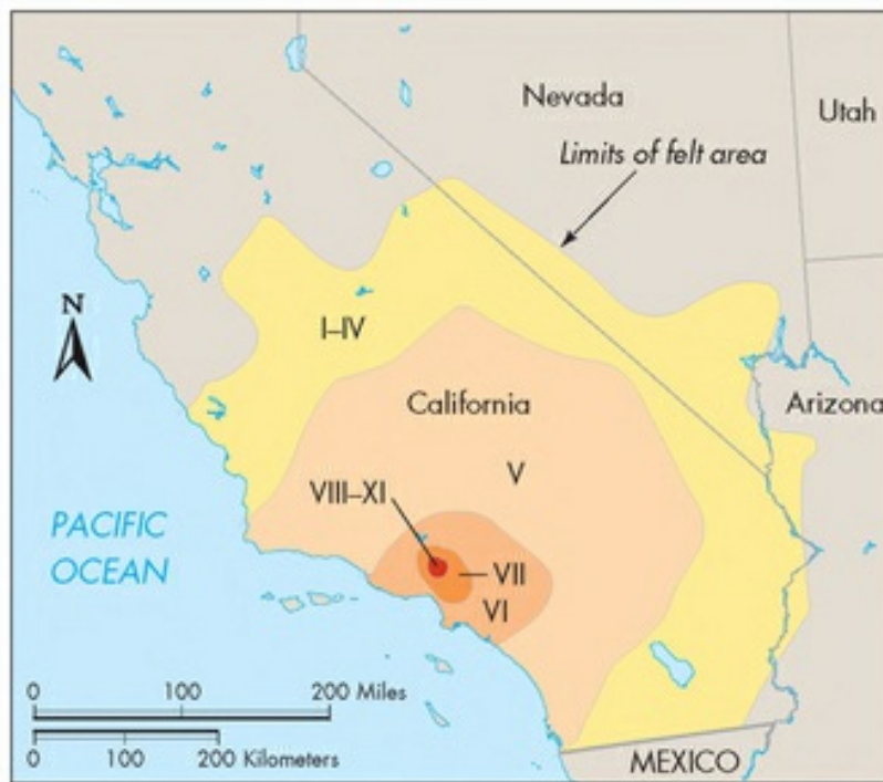
FIGURE 3.12 Intensity of Shaking Modified Mercalli Intensity map for the 1971 Sylmar, California, earthquake (M 6.7), determined after the earthquake. The red and orange areas experienced the most intense shaking. See Table 3.4 for an explanation of the Roman numerals. (U.S. Geological Survey, 1974. Earthquake Information Bulletin 6[5])
