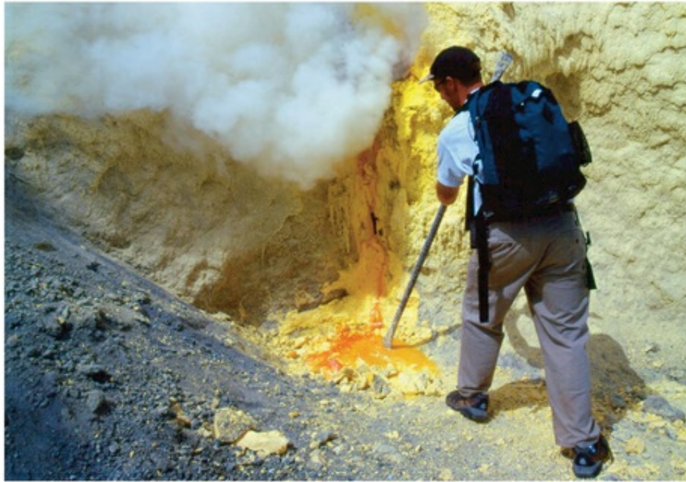
FIGURE 5.4.A Volcanologist Sampling Molten Sulfur Volcanologist Chris Eisinger uses a crowbar to hit some molten sulfur on Kawah Ijen volcano in Indonesia. The 200°C (~390°F) molten sulfur is still red hot and will cool to a yellow or green color. (Chris Eisinger)
