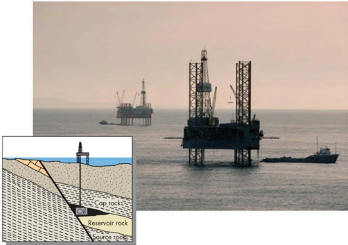
FIGURE 1.15 Hydrocarbon Trap Faulting in the Santa Barbara Channel has produced a linear fault trap, along which oil rigs at the surface are situated above. (Nik Wheeler/Corbis)
