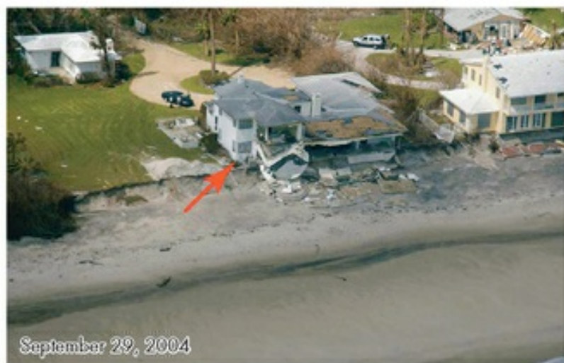
FIGURE 11.15 Storms Contribute to Coastal Erosion Two hurricanes, 21 days apart, eroded sand from this coastline in Vero Beach on Florida's east coast. The top picture, taken in August 1997 before the hurricanes, shows a sand dune providing some protection for the homes. In the middle picture, taken on September 8, 2004, after Hurricane Frances, the dune has migrated next to the houses. The third picture, taken on September 29, 2004, after Hurricane Jeanne,
